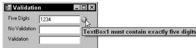
Figure 2-20: The Validating event fires when the focus moves to a control that has CausesValidation set to True .
