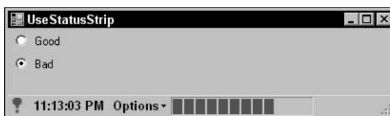
Figure G-22: The StatusStrip control allows a program to display status information.
