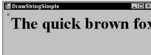
Figure 21-1: Text doesn't begin exactly at the starting point passed to the DrawString method.
