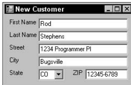
Figure 2-15: This dialog uses Anchor properties to make its TextBox controls use whatever space is available on the form.
