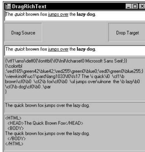
Figure 13-1: This program drags and drops data in Text, Rtf, and Html formats.
