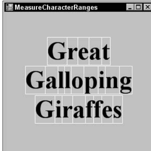
Figure 21-10: The Graphics object's MeasureCharacterRanges method shows where ranges of characters will be drawn in a string.
