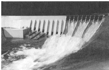
■ FIGURE 7.8 A scale hydraulic model (1:197) of the Guri Dam in Venezuela which is used to simulate the characteristics of the flow over and below the spillway and the erosion below the spillway. (Photograph courtesy of St. Anthony Falls Hydraulic Laboratory.)
