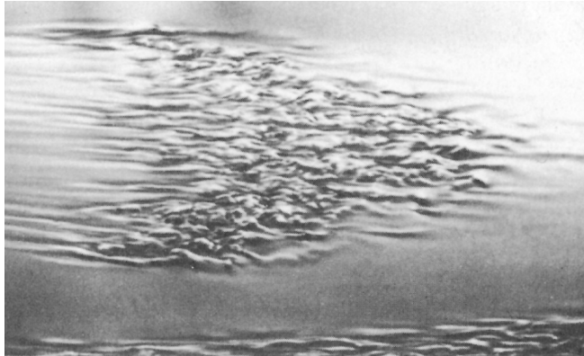
■ FIGURE 9.13 Turbulent spots and the transition from laminar to turbulent boundary layer flow on a flat plate. Flow from left to right. (Photograph courtesy of B. Cantwell, Stanford University.)
