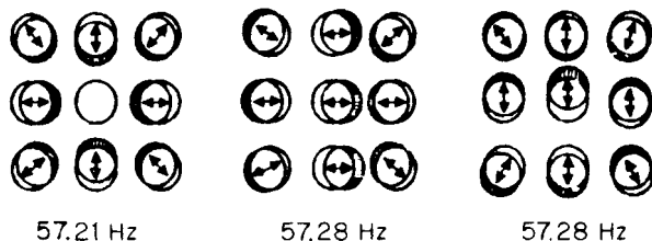
FIGURE 29.5 Coupled modes of vibration of a bank of tubes in a dense fluid. 6
