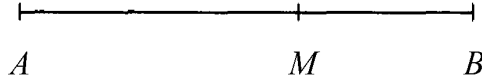
FIGURE B.1 . Definition of the golden section. If [AB] : [AM] = [AM] : [MB] , then \phi = [AM] : [MB] .
