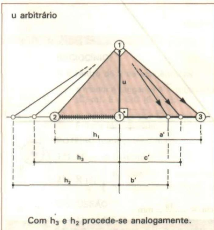
$$\left. \begin{aligned} u^2 &= h_1 \cdot a' \Rightarrow a' = \frac{u^2}{h_1} \\ u^2 &= h_2 \cdot b' \Rightarrow b' = \frac{u^2}{h_2} \\ u^2 &= h_3 \cdot c' \Rightarrow c' = \frac{u^2}{h_3} \end{aligned} \right\} (**)$$
