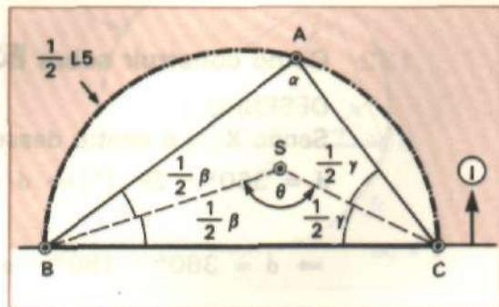
$$\begin{aligned} \text{No } \triangle SBC : \theta &= 180^\circ - \left( \frac{\beta}{2} + \frac{\gamma}{2} \right) = 180^\circ - \frac{\beta + \gamma}{2} \\ \text{No } \triangle ABC : \beta + \gamma &= 180^\circ - \alpha \end{aligned} \Rightarrow \theta = 180^\circ - \frac{180^\circ - \alpha}{2}$$
