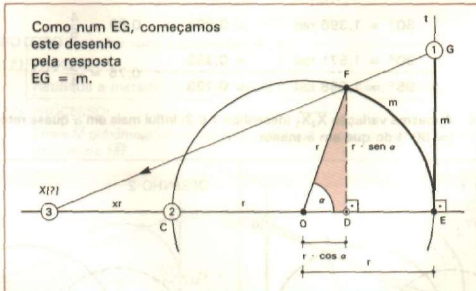
$$\begin{aligned} 2\pi r &= 2\pi \text{ rad.} \therefore \\ m &= \alpha \\ \text{logo:} \\ \alpha &= \frac{m \cdot 2\pi \text{ rad}}{2\pi \cdot r} \\ m &= r \cdot \alpha \end{aligned}$$
