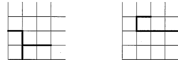
Figure 12.6 Two examples of bond clusters. The occupied bonds are shown as bold lines.
