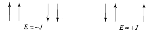
Figure 15.1 The interaction energy between nearest neighbor spins in the absence of an external magnetic field.
