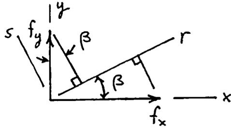
$$\begin{aligned} f_r &= f_x \cos \beta + f_y \sin \beta \\ f_s &= -f_x \sin \beta + f_y \cos \beta \end{aligned} \quad \text{or} \quad \begin{Bmatrix} f_r \\ f_s \end{Bmatrix} = \underbrace{\begin{bmatrix} \cos \beta & \sin \beta \\ -\sin \beta & \cos \beta \end{bmatrix}}_{[\tilde{\Lambda}]} \begin{Bmatrix} f_x \\ f_y \end{Bmatrix}$$
