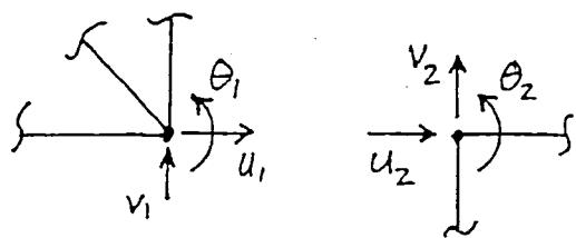
$$\begin{bmatrix} -1 & 0 & 0 & 0 & 1 & 0 \\ 0 & -1 & 0 & 0 & 0 & 1 \end{bmatrix} \begin{bmatrix} u_1 \\ v_1 \\ \theta_1 \\ u_2 \\ v_2 \\ \theta_2 \end{bmatrix} = \{0\}$$
