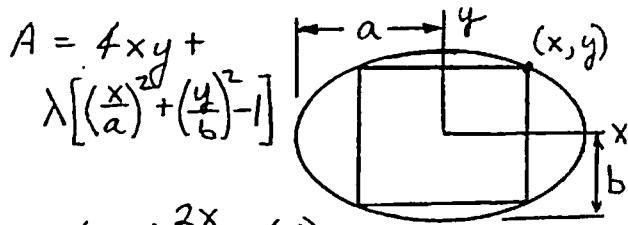
$$\frac{\partial A}{\partial x} = 0 = 4y + \lambda \frac{2x}{a^2} \quad (a)$$
