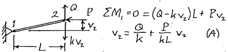
$$v_2 = \frac{Q}{k} + \frac{P}{kL} v_2 \quad (A)$$
