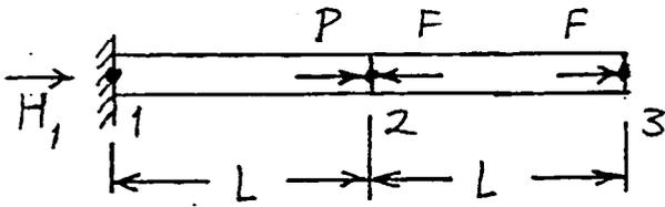
$$\sigma_0 = -E\alpha \frac{T_2 + T_3}{2} \quad (\text{right element only})$$
