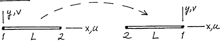
$$[u_1 \quad v_1 \quad \theta_{z1} \quad u_2 \quad v_2 \quad \theta_{z2}] = [0 \quad 0 \quad \pi \quad -2L \quad 0 \quad \pi]$$
