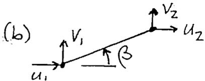
$$\{d\} = [c_1 \ c_2 \ c_1 - c_3 L \sin \beta \ c_2 + c_3 L \cos \beta]^T$$
