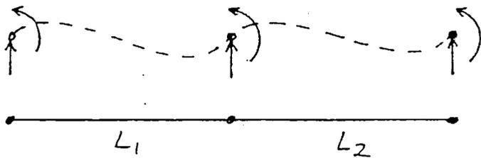
Direction of middle force arrow is upward, as shown, if  $L_1 > L_2$ .
