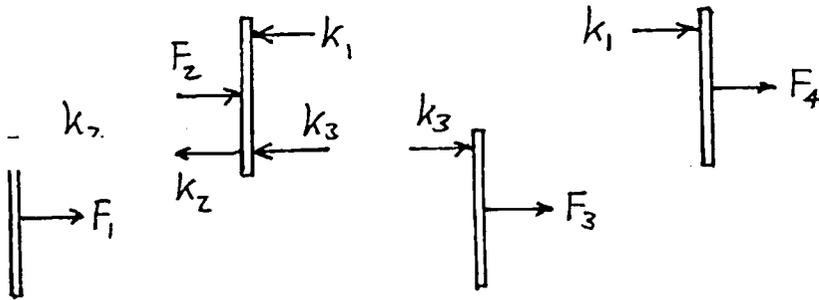
**2.2-3** Activate d.o.f. in turn to unit value; each time calculate loads that therefore must be applied to the two d.o.f.
