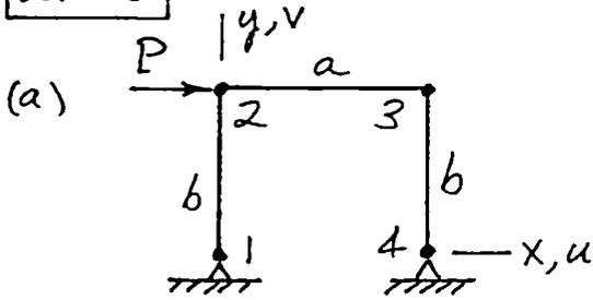
$$AE \begin{bmatrix} 1/a & 0 & -1/a & 0 \\ 0 & 1/b & 0 & 0 \\ -1/a & 0 & 1/a & 0 \\ 0 & 0 & 0 & 1/b \end{bmatrix} \begin{Bmatrix} u_2 \\ v_2 \\ u_3 \\ v_3 \end{Bmatrix} = \begin{Bmatrix} P \\ 0 \\ 0 \\ 0 \end{Bmatrix}$$
