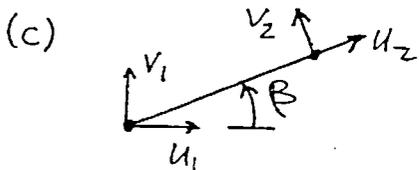
$$\{d\} = [c_1 \ c_2 \ c_1 \cos \beta + c_2 \sin \beta \ -c_1 \sin \beta + c_2 \cos \beta + c_3 L]^T$$
