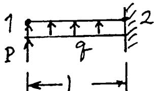
$$\begin{bmatrix} L/3EI & -1/L \\ -1/L & 0 \end{bmatrix} \begin{Bmatrix} M_2 \\ v_1 \end{Bmatrix} = \begin{Bmatrix} 0 \\ -P - qL/2 \end{Bmatrix}$$
