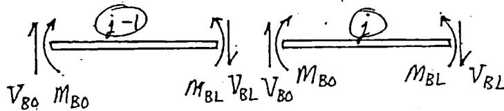
Consider e.g. assembly of vertical forces where elements  $j-1$  and  $j$  meet. The dashed line connects forces having the same global d.o.f. number. These add, to yield the net force  $(V_{BO})_j - (V_{BL})_{j-1}$  at the shared node.
