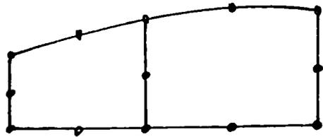
Hence on a common edge such as this, the field quantity is defined by the same three nodal d.o.f. and uses the same  $N_i$  whether viewed from the left element or the right, so the identical curve  $\phi = \phi(\eta)$  is produced.
