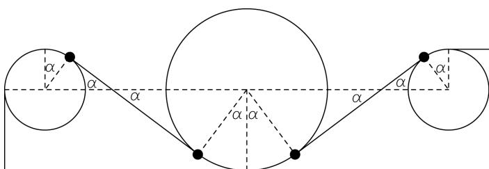
To determine the angle  $\alpha$ , part of the diagram is shown here with the radii of the circles marked.
