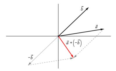
As we can see from this figure we can move the vector representing  $\vec{a} + (-\vec{b})$  to the position we've got in the first figure showing the difference of the two vectors.
