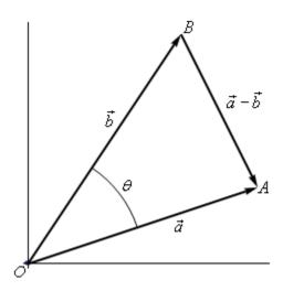
The three vectors above form the triangle *AOB* and note that the length of each side is nothing more than the magnitude of the vector forming that side.
