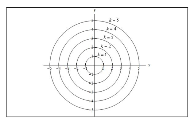
Note that we can think of contours in terms of the intersection of the surface that is given by z = f(x, y) and the plane z = k. The contour will represent the intersection of the surface and the plane.
