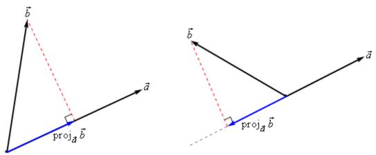
So, to get the projection of  $\vec{b}$  onto  $\vec{a}$  we drop straight down from the end of  $\vec{b}$  until we hit (and form a right angle) with the line that is parallel to  $\vec{a}$ . The projection is then the vector that is parallel to  $\vec{a}$ , starts at the same point both of the original vectors started at and ends where the dashed line hits the line parallel to  $\vec{a}$ .
