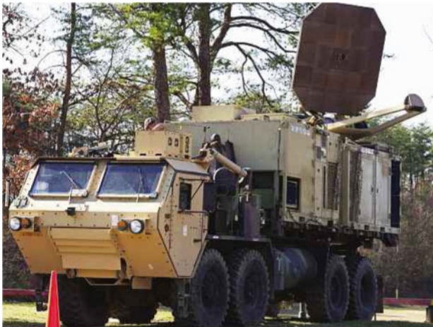
LEFT: The Active Denial system mounted on a US Marine Corps truck. RIGHT: A TV reporter reacts as he is targeted by the system.
