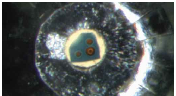
LEFT: A crystal of blue ringwoodite being crushed in a lab experiment.
