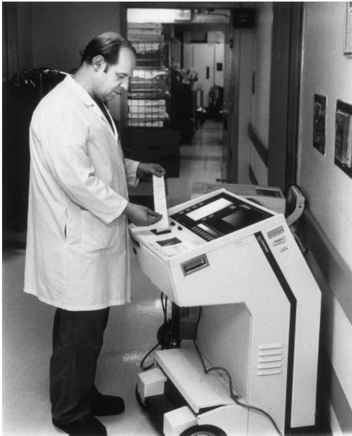
Figure 4. Emergency support, balloon pump. Clinical engineering plays a key role in providing emergency support to troubleshoot and answer questions relating to equipment operation and capability. Here a clinical engineer is running a test to assure that a balloon pump located outside a Cath-Lab is functioning properly. This device provides support to critically ill patients by reducing their heart's workload until it strengthens. Balloon inflate/deflate timing and mode of triggering assure optimal patient assistance.
