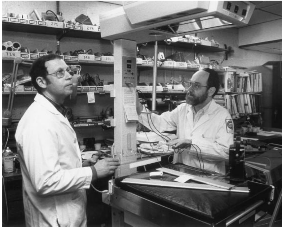
Figure 11. Repair, infant warmer. Repair of medical instrumentation requires electrical troubleshooting skills. Here, an infant warmer is being evaluated using a multimeter to assure that the thermostat controls will function properly so as to prevent harm to the infants.
