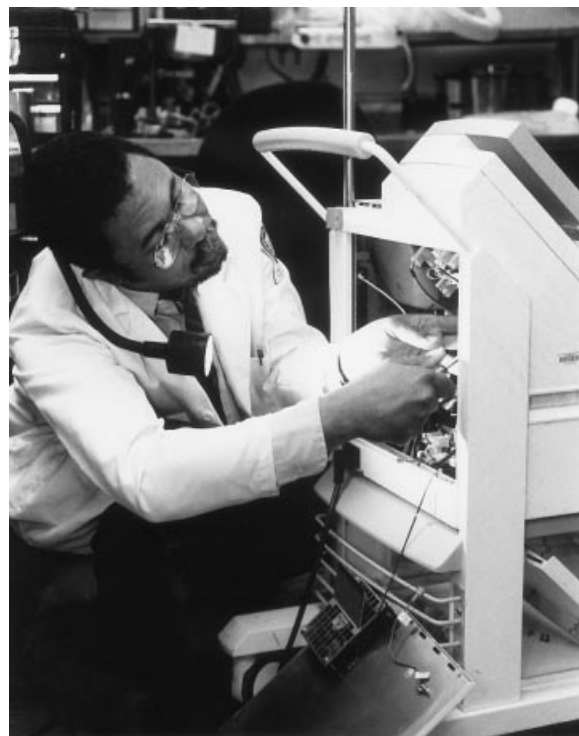
Figure 10. Preventive maintenance cell saver. Depending on the medical instrument, preventive maintenance can be more involved than just a functional and safety test. Problems that are uncovered must be rectified, and some instrumentation requires that components be replaced due to wear or number of hours of use. This, as well as observed spills, may necessitate opening the unit. The cell saver shown is used to salvage blood shed during an operation allowing its return to the same patient.
