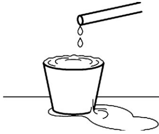
Figure 3. Mechanical example of a relaxation oscillator.
