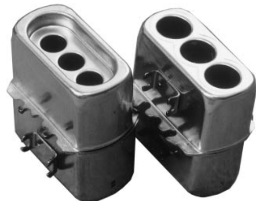
Figure 18. Photograph of grids creating the low-voltage side of the main focus lens illustrating the expanded lens type of grid on the left and showing a conventional three-lens type of grid on the right.
