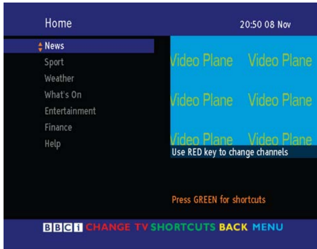
Figure 8. Introduction Page for Digital Teletext (in practice the section shown as 'Video Plane' will contain a reduced-size version of the TV program video).
