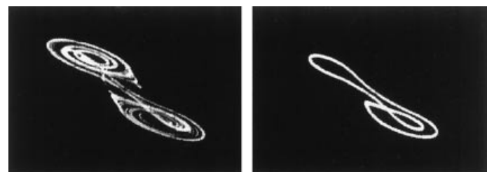
Figure 10. The double scroll attractor can be eliminated and the behavior converted to one of the periodic orbits in experiments in the delayed feedback control of Chua's circuit.
