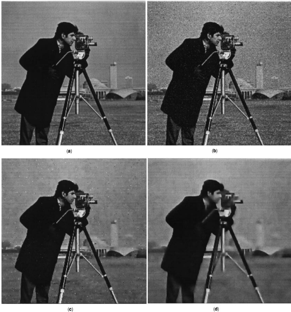
Fig. 4. (a) Original “Cameraman” image. (b) “Cameraman” image corrupted with additive Laplacian-distributed noise. (c) After eight iterations of anisotropic diffusion with diffusion coefficient in Eq. (21). (d) After eight iterations of anisotropic diffusion with diffusion coefficient in Eq. (22).
