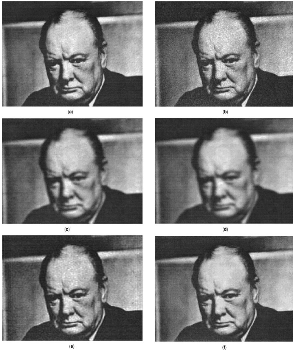
Fig. 2. (a) Original “Winston” image. (b) Corrupted “Winston” image with additive Gaussian-distributed noise ( \sigma = 10 ). (c) Average filter result ( 5 \times 5 window). (d) Gaussian filter result (standard deviation \sigma = 2 ). (e) Ideal low-pass filter result (cutoff = N/4 ). (f) Wavelet shrinkage result.
