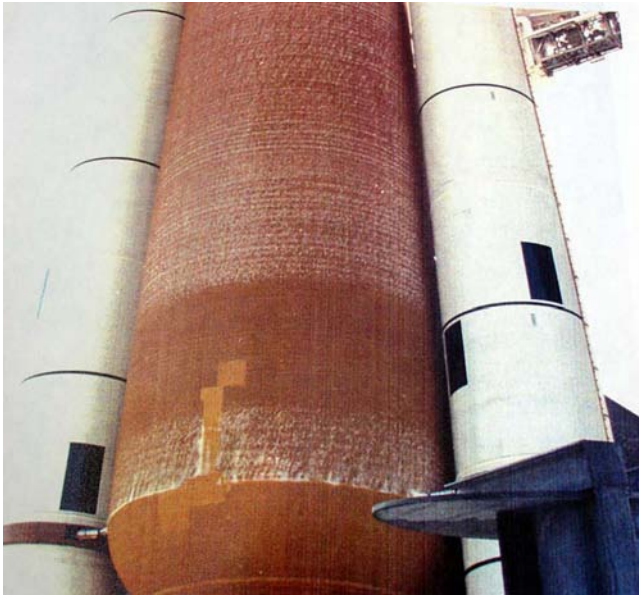
Figure 25. Frost and ice on the space shuttle ET SOFI (Courtesy of NASA KSC).
