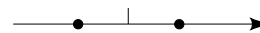
Figure 4. An uncoded BPSK constellation. Each point represents a signal to be transmitted over the channel.
