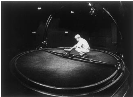
Figure 6. The EGO goniometer installed at JRC, Ispra, Italy.
