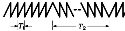
Figure 5. The input signal of a sawtooth wave test is derived from inverting the phase of a 30 kHz sawtooth waveform with a 30 kHz/256 period. T_1 = 1/30 kHz, T_2 = 256T_1 .
