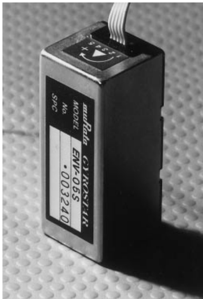
Figure 8. The Gyrostar manufactured by Murata Electronics. This is a small, relatively inexpensive, single-axis piezoelectric rate gyroscope originally developed for the automobile market and active suspension systems. (See B. Barshan and H. F. Durrant-Whyte, IEEE Trans. Robot. Automa. 11 (3), 328–342, June 1995. Copyright IEEE, 1995.)
