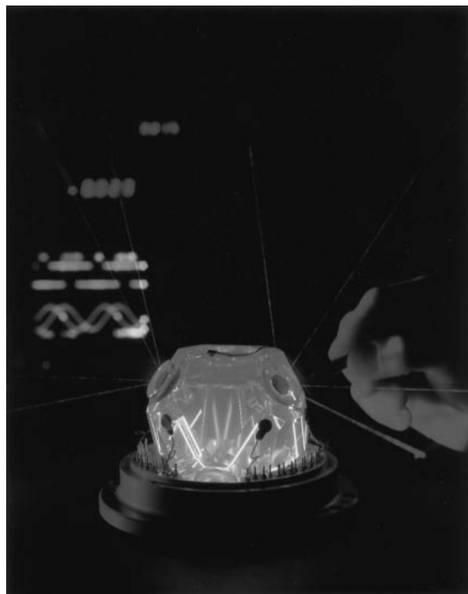
Figure 13. An example triaxial monolithic RLG operating at 632.8 nm. (Photo courtesy of Kearfott Guidance & Navigation Corporation, Inc., Wayne, NJ.)
