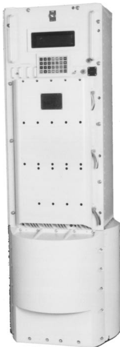
Figure 2. MK-49 ring laser gyro navigator by Sperry Marine Inc. This is a navigational quality gyroscope. (Photo courtesy of Sperry Marine Inc., Charlottesville, VA.)
