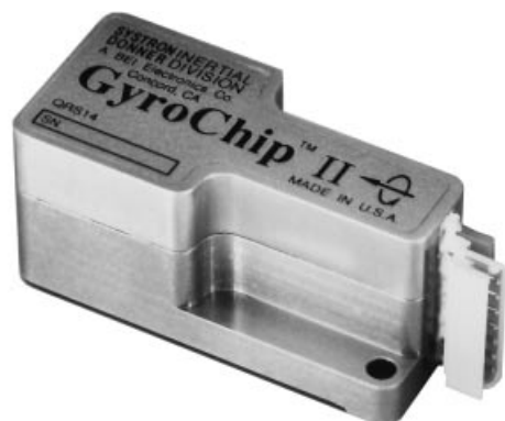
Figure 6. The GyroChip II solid-state gyro which employs a quartz tuning fork. Several thousand of these items can be mass-produced in a single batch. (Photo courtesy of Systron Donner Inertial Division, Concord, CA.)
