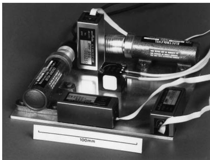
Figure 22. A low-cost INS comprising three gyroscopes, a triaxial accelerometer and two tilt sensors, developed for a mobile robot platform. (See B. Barshan and H. F. Durrant-Whyte, IEEE Trans. Robot. Automa. 11 (3), 328–342, June 1995. Copyright IEEE, 1995.)
