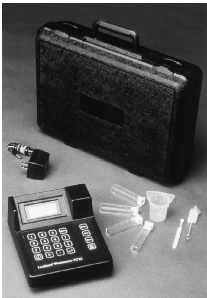
Figure 9. A single-channel, microprocessor-controlled photometer used to measure impurities in water. The transparent cells shown on the right each hold 10 ml of water and reagent. (Courtesy of VWR Scientific Products.)
