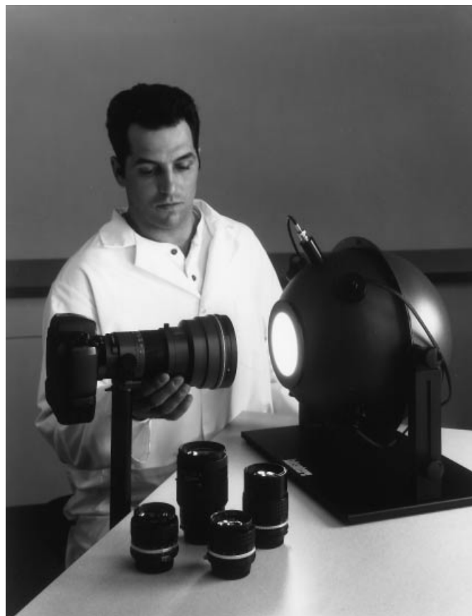
Figure 13. Integrating sphere uniform source for luminance calibration of photometers and imaging systems. (Courtesy of Labsphere Inc., North Sutton, NH)
