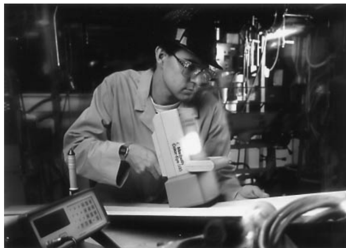
Figure 10. Portable, dual-beam, array detector spectrophotometer used for making precision color measurements. The sample material is illuminated by a pulsed-Xe lamp built into the instrument. (Courtesy of GretagMacbeth, © 1998. GretagMacbeth™ is a trademark of GretagMacbeth LLC. All rights reserved. Color-Eye® is a registered trademark of GretagMacbeth LLC. All rights reserved.)
