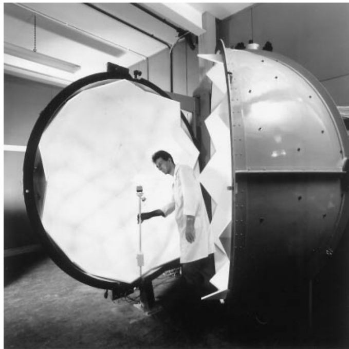
Figure 7. Two-meter-diameter integrating sphere photometer. (Courtesy of the UK's National Physical Laboratory. Copyright © Crown 1998. Reproduced by permission of the Controller of HMSO.)
