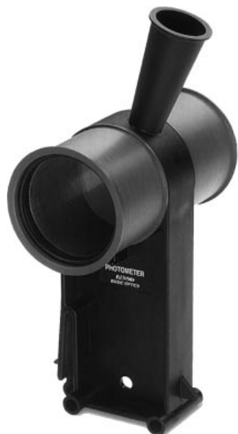
Figure 3. A commercially available bench photometer. The photometer is moved in relation to the two light sources located near the ends of an optical bench until equal brightness on two fluorescent disks is observed through the eyepiece. (Courtesy of PASCO scientific.)
