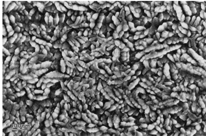
Figure 31. High-resolution image of magnetic disk media surface recorded at 30 keV in a JEOL JSM 890 field-emission SEM. [Courtesy D. Joy (19).]
