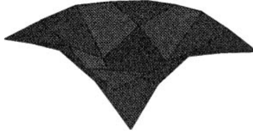
Fig. 8. Digital realization of the Laplacian of Gaussian using a difference of Gaussian approach. The masks of Fig. 7 are used.
