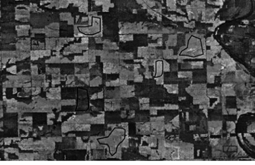
Figure 4. Delineation of training sites on the computer screen. The analyst must have definite knowledge about the areas to represent and the training sites must be carefully delineated inside homogenous fields to avoid inclusion of pixels (i.e., mixed or polluted pixels) from other categories surrounding the area under consideration. These training sites will train the classifying algorithm to recognize the spectral signature of each category; and “bad” training will confuse the algorithm and result in misclassification (from Lillesand and Kiefer, Ref. 4).
