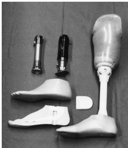
Figure 4. Lower limb prosthetic componentry. Two pylons (an aluminum shank and a hydraulic shank), two feet (a SACH foot and a Seattle foot that has been sectioned to show the plastic leaf spring), a heel wedge, and an assembled transradial amputee prosthesis are shown.
