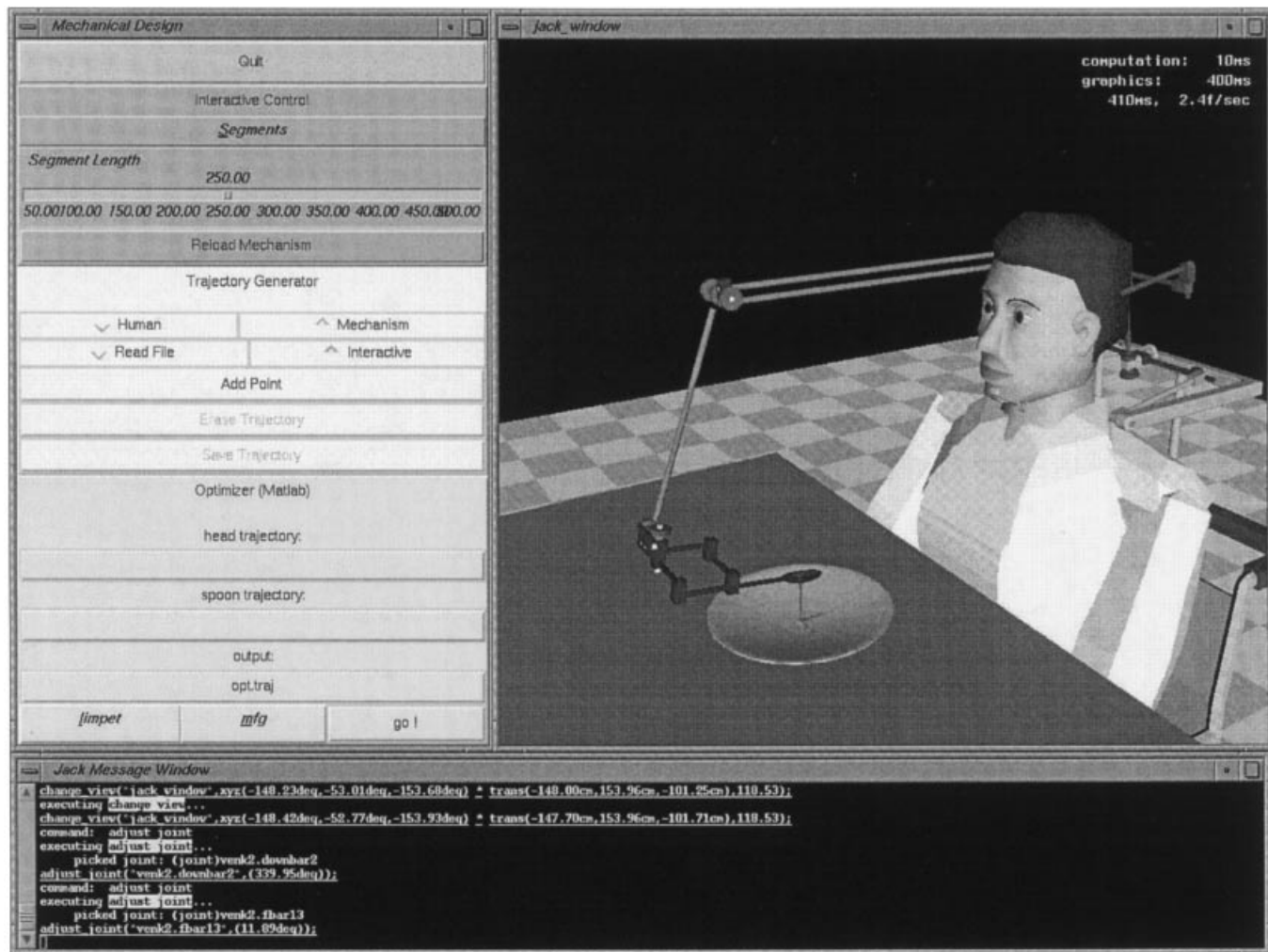
Figure 9. The central virtual user interface for visualization and optimization of the design.
