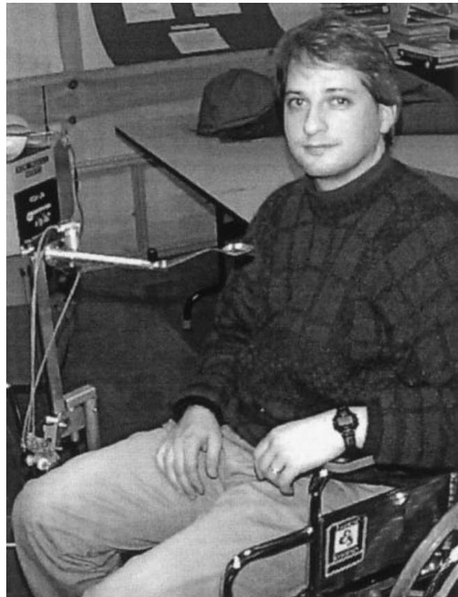
Figure 3. An articulated mechanism for feeding in a foot-controlled feeding device (Magpie) designed at the Nuffield Orthopaedic Center in Oxford, England (75).
