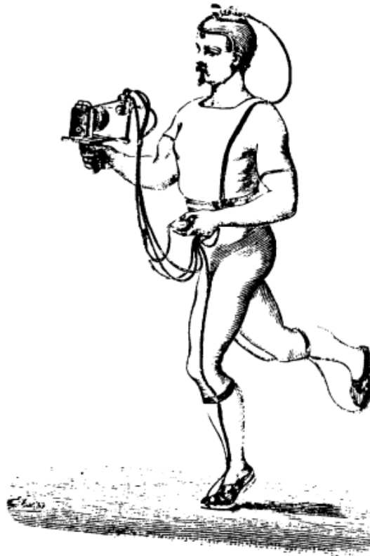
Fig. 1. The recording mechanism developed by É. J. Marey to study human locomotion. From Marey (37).
