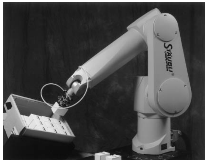
Figure 1. Packaging and palletizing operation with a Staubli Unimation robot. Courtesy of Staubli Corporation, Duncan, SC.
