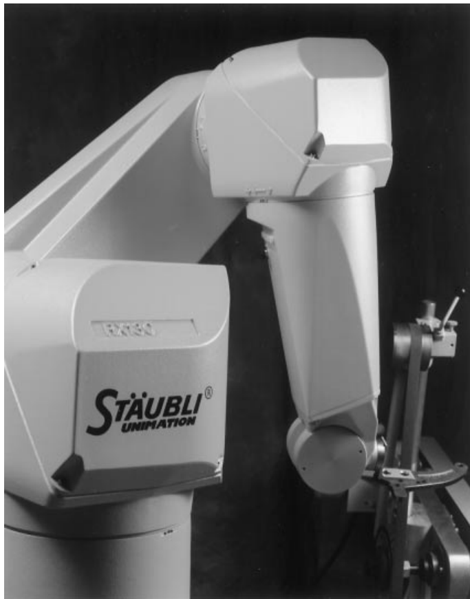
Figure 17. Stäubli Unimation RX 130 robot in a compound angle deburring operation. Courtesy of Stäubli Corporation, Duncan, SC.
