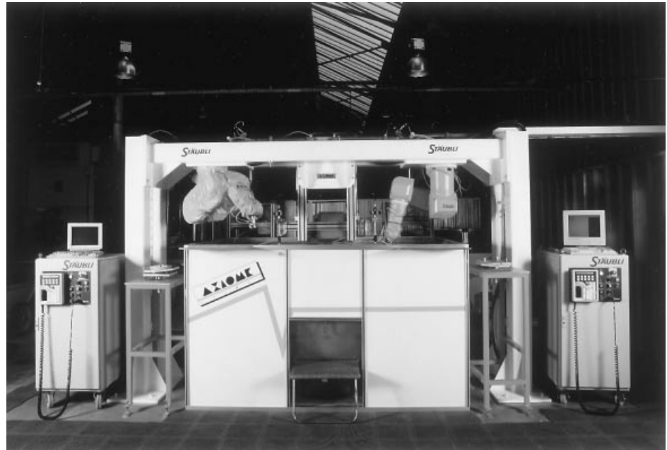
Figure 16. Stäubli waterjet cutting system setup. Courtesy of Stäubli Corporation, Duncan, SC.
