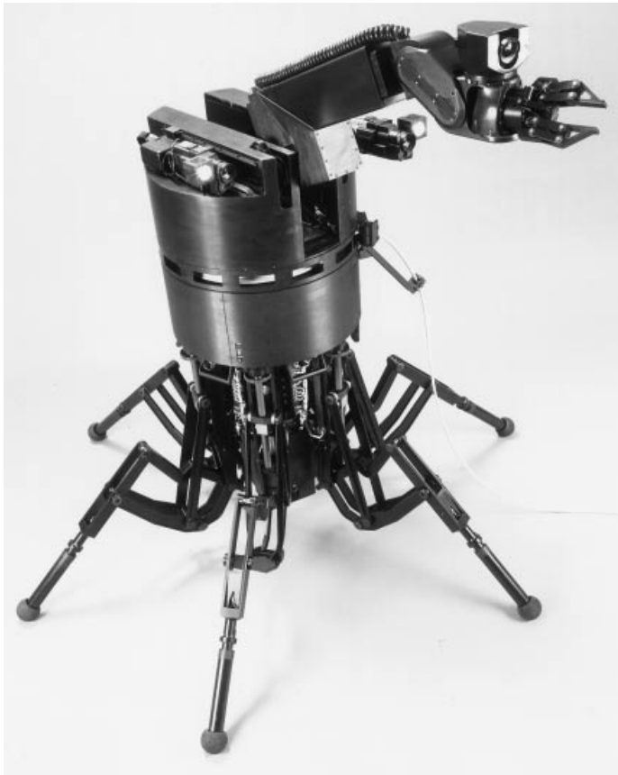
Figure 9. Odex II, A walking robot that can support up to (50 lb). Courtesy of Odetics, Inc., Anaheim, CA.
