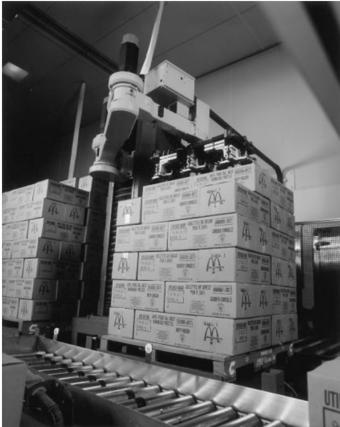
Figure 5. Robotic case palletizing of frozen meat patties with an M-400 robot from Fanuc Robotics. Courtesy of Fanuc Robotics.
