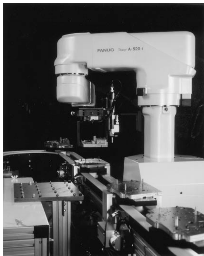
Figure 9. Robotic assembly of a valve body housing with A-520 i robot. Courtesy of FANUC Robotics North America, Inc.
