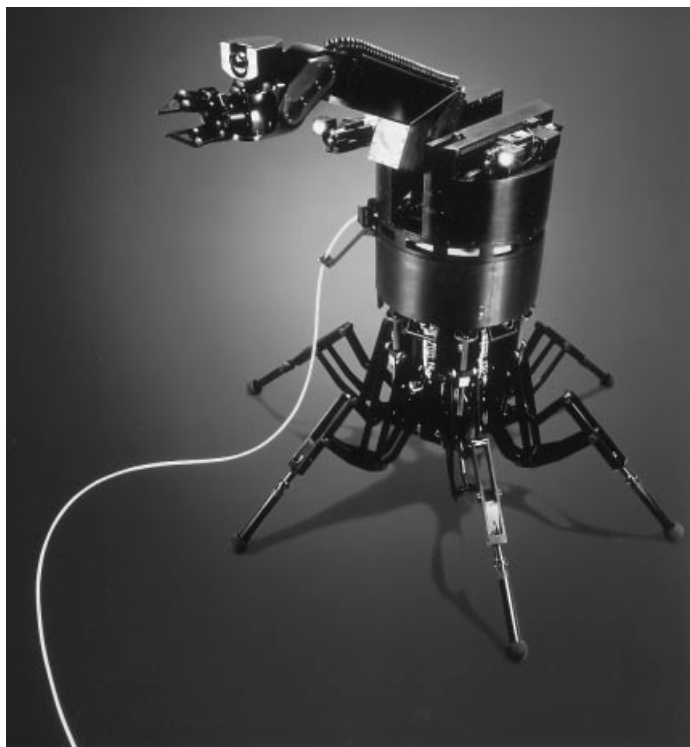
Figure 11. Odex II incorporates full-force reflection feedback in the articulator leg assemblies. Courtesy of Odetics, Anaheim, CA.
