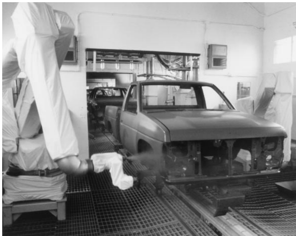
Figure 8. Automotive spray painting with P-200 robot system. Courtesy of FANUC Robotics North America, Inc.
