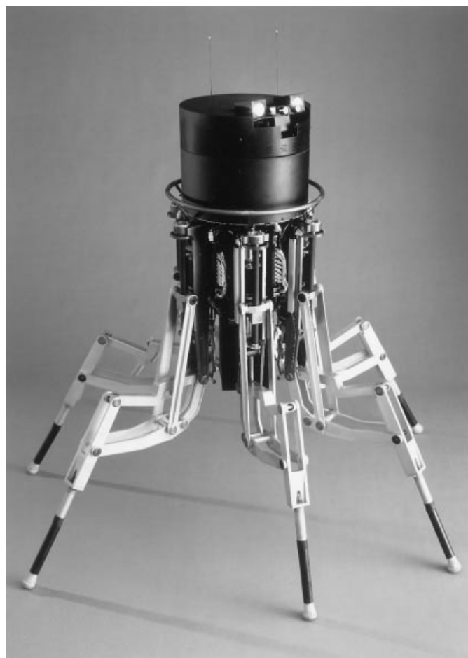
Figure 12. Odex I uses video cameras for transmitting imagery to a remote human operator. Courtesy of Odetics, Anaheim, CA.
