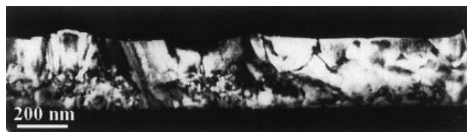
Figure 16. Cross-sectional view of a 160 nm thick polysilicon film sequentially annealed by SPC at 600°C for 12 h and subsequently by ELC at 350 mJ/cm 2 . It is evident that in the upper part of the film (where the primary melt induced by the laser irradiation occurs) a much lower defect density is present (courtesy of J. Stoemenos).
