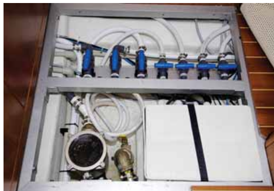
THE NAV STATION DOUBLES as an entertainment center. When it's time to plot, the flat-screen monitor comes out from the bulkhead on an articulating arm. The boat's plumbing, which is accessed under a removable floorboard in the main salon, is clearly labeled. Deep bilges, and an aluminum framework that supports the floorboards are hallmarks of Nautor's Swan builds.
