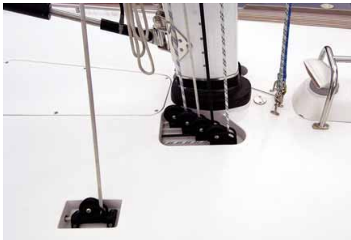
ALL SAIL HANDLING CONTROLS ON THE SWAN 46, including halyards, cunningham, and reefing lines are led aft from the mast to the cockpit under the deck. The mainsheet (outboard) is also led underdeck. Note the access panel to the halyards aft of the mast.
