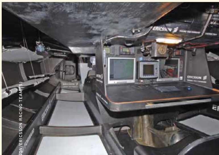
Looking forward from the aft watertight bulkhead, the nav station is at right. Forward, and underneath the companionway stairs is the dedicated media station. Note how every surface is rounded, which makes moving sails from side to side easier.
