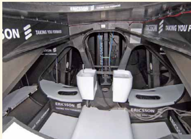
The view from the companionway shows the working area of the boat. At center is the galley, and outboard are panels covering the hydraulic keel cylinders. Inspection ports allow them to see the keel's position. Behind the mast is a solid wall enclosing the head.
